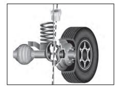
**Tech Tip:** Some Ford trucks come from the factory with an offset bushing already installed. Not all these bushings are clearly marked. By installing a 0° bushing first, you eliminate math errors when calculating the proper adjustment needed.
